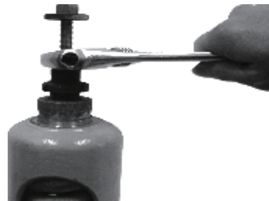
Fig. 8 Adjustment method of set pressure
